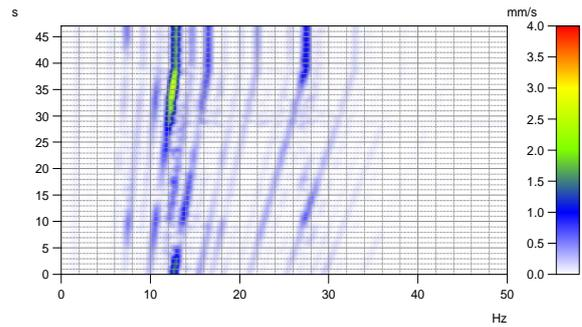
Figure 11: Time-frequency-amplitude spectrum of the calculated vibrational velocity in y-direction at node 244 (max. 3.1 mm/s rms) excitation in y-direction, rotational sweep 90 – 110 rpm.
