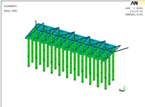
Figure 7: FEM-model of the 2<sup>nd</sup> design of reciprocating pump foundation, connection of the slab of the pump house to the massive drilling cellar by framework construction.
