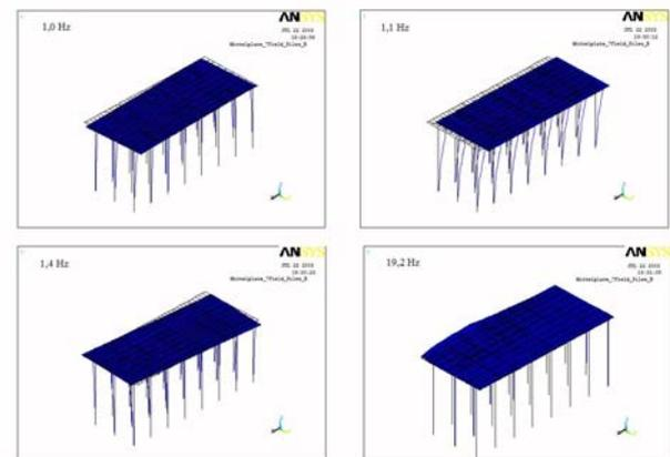
Figure 5: Natural mode shapes of the first design of the pump installation, undeformed: unfilled grid, deformed: filled grid.
