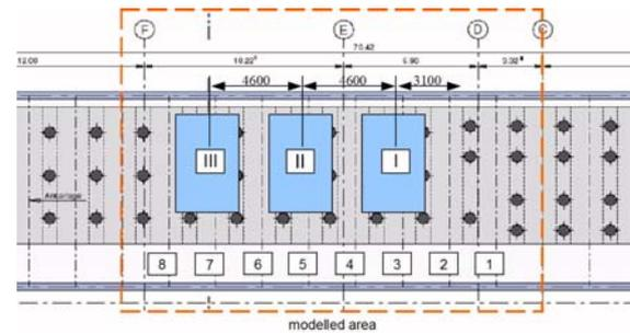
Figure 4: Positions of the mud pumps and alignment of the piles, first design.
